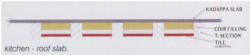
Fig. 38. Section of the roof of kitchen
