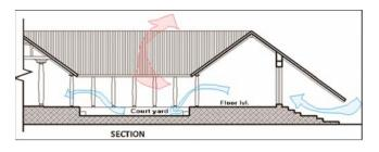
Fig. 7—Courtyard, minimum openings and projected eaves reduce the solar heat gain and regulate the air flow through the building.
